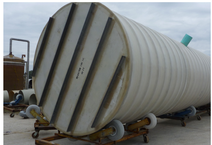
▼ WETWELL BOTTOM WITH STRUCTURAL ANCHORS
