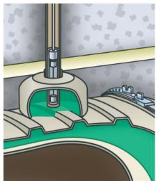
Hydrostatically Monitored Double-Wall Fiberglass Tank Sump
